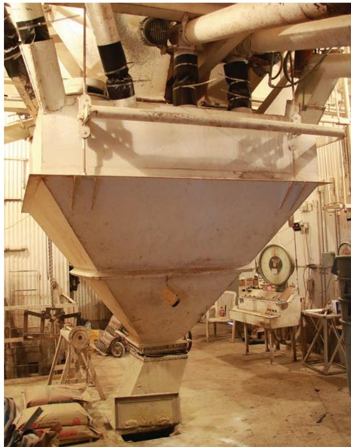
*The main batch hopper inside the mill is used to mix the ingredients that make up the feed.*
